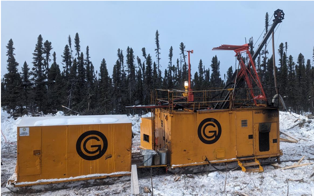
Figure 2: Diamond drill rig at Horden Lake project
