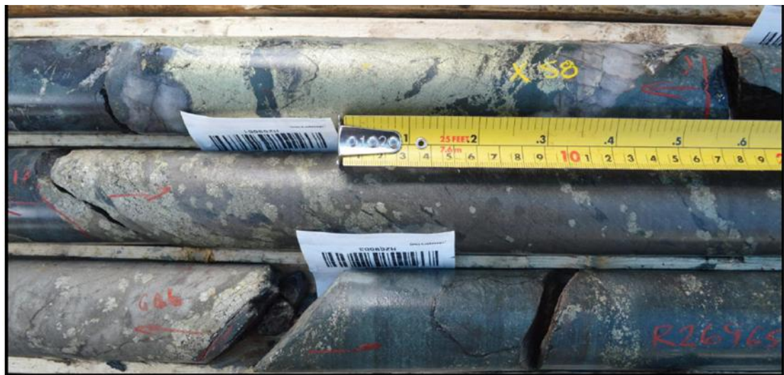
Figure 4: Massive chalcopyrite and massive pyrrhotite with coarse pyrite. Allotta occurrences drill hole 20-ZA-05, composite 57.00-62.30m. Refer Table 1 for assay results.
