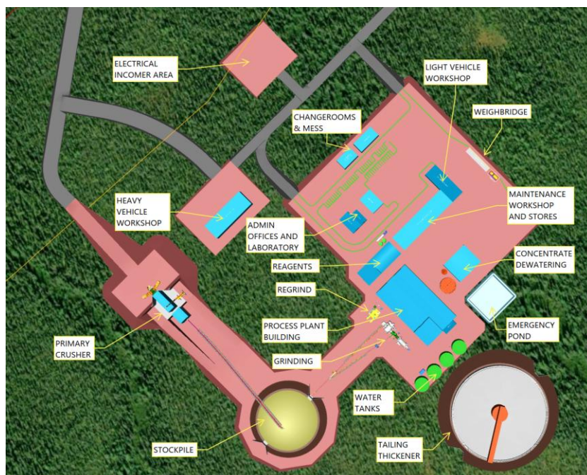
Figure 9: Horden Lake process plant layout
